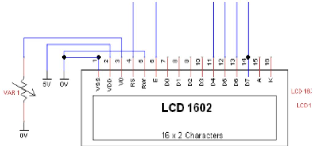
Fig 1.4: LCD Display Unit
