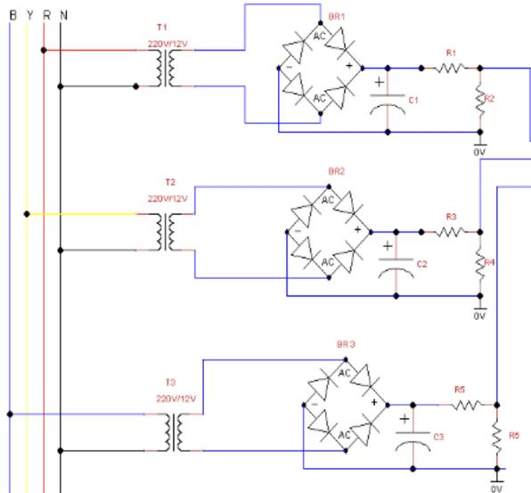
Fig. 1.2: Circuitry of 3-Phase Sensing Unit
