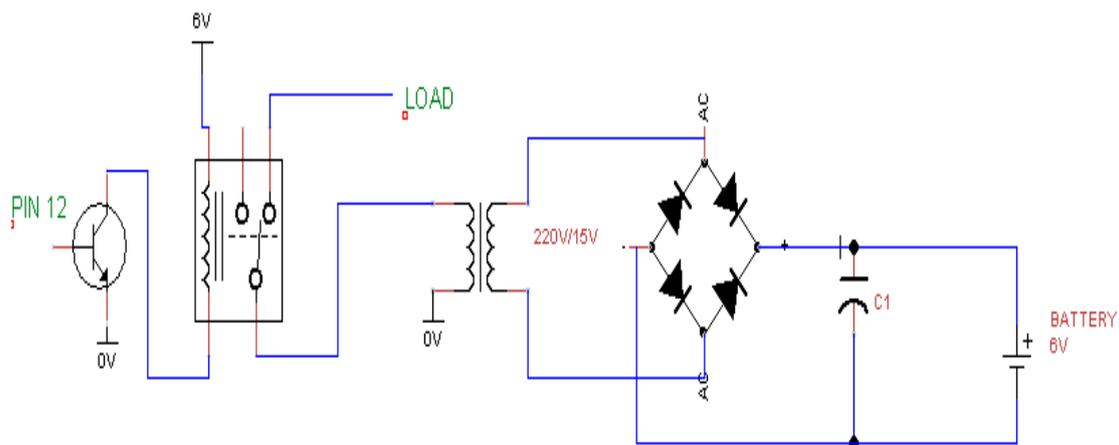
Fig. 1.5: Circuit diagram for the Power bank module
