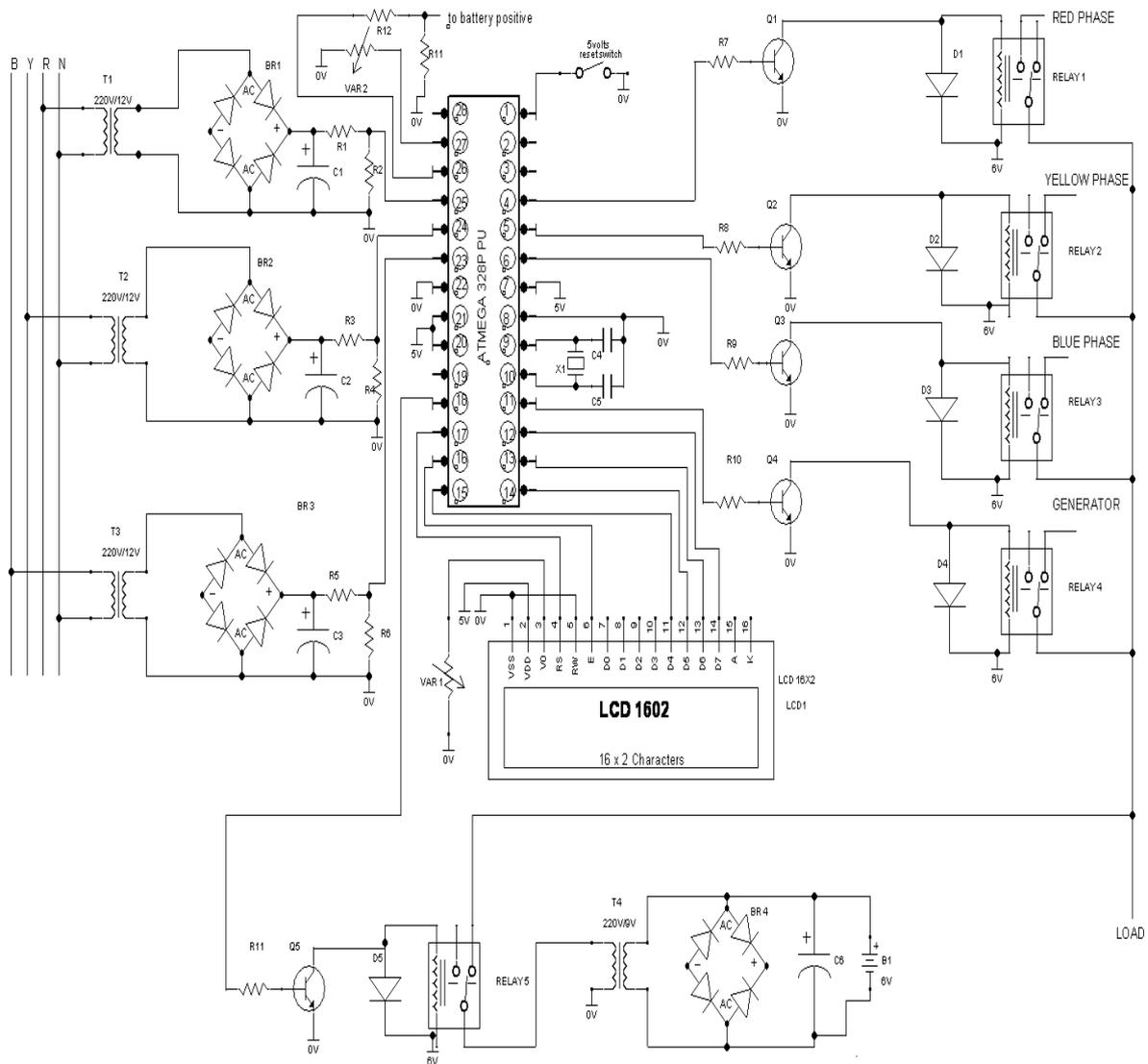
Fig. 1.7: Circuit diagram of the Automatic Phase Selector and Changeover Switch
