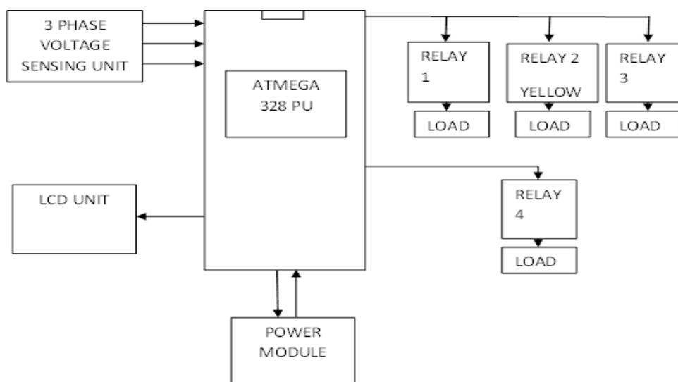
Figure 1.1: Block diagram of Automatic Phase Selector and Changeover Switch
